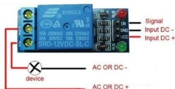
Gambar 10. Modul Relay Normally Close
