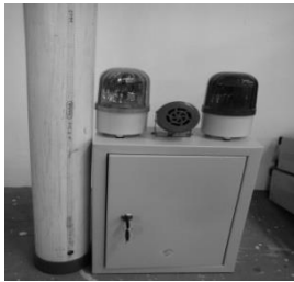
Gambar 5. Sistem Deteksi Dini Banjir Berbasis Sensor Float Magnetic Level Gauge
