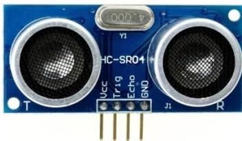
Gambar 2. Sensor Ultrasonik HC-SR04
