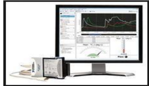
Gambar 4 Data Logger Berbasis PC (Sumber: Yanuar Rachmatefendi, 2018)
