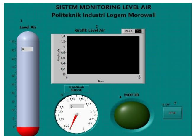
**Gambar 6.** Tampilan Sistem Monitoring LabVIEW
