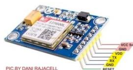
**Gambar 5.** Modul GSM SIM 800Lv2
