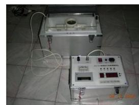
Gambar 2 Breakdown Voltage Test Machine
