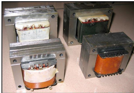
Gambar 5. Transformator Step-Down (Sumber : Andrianto, 2015)
